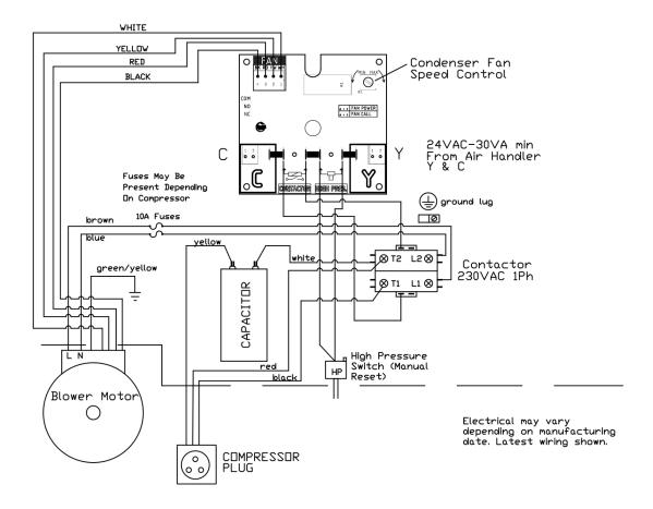
This diagram is provided as reference only. Wiring may differ depending on the unit. Always refer to correct wiring diagram located on inside cover of electrical panel
